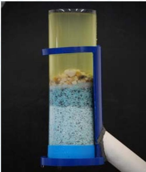
The media absorbs the oil, forming a seal that prevents any oil from discharging.
