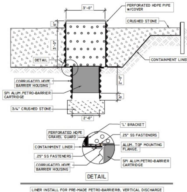
In some installations using concrete, crushed stone is not used so the gravel guard is not required. In those applications only the Top-Hat-Filter is used. When No crushed stone is used in the containment area.
