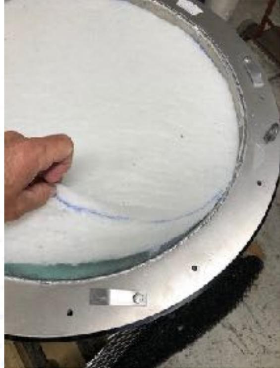
Next filter is 2" thick polyester batting which collects the finer dirt. The top layers can be removed until the complete batting is dirty and requires replacement.
